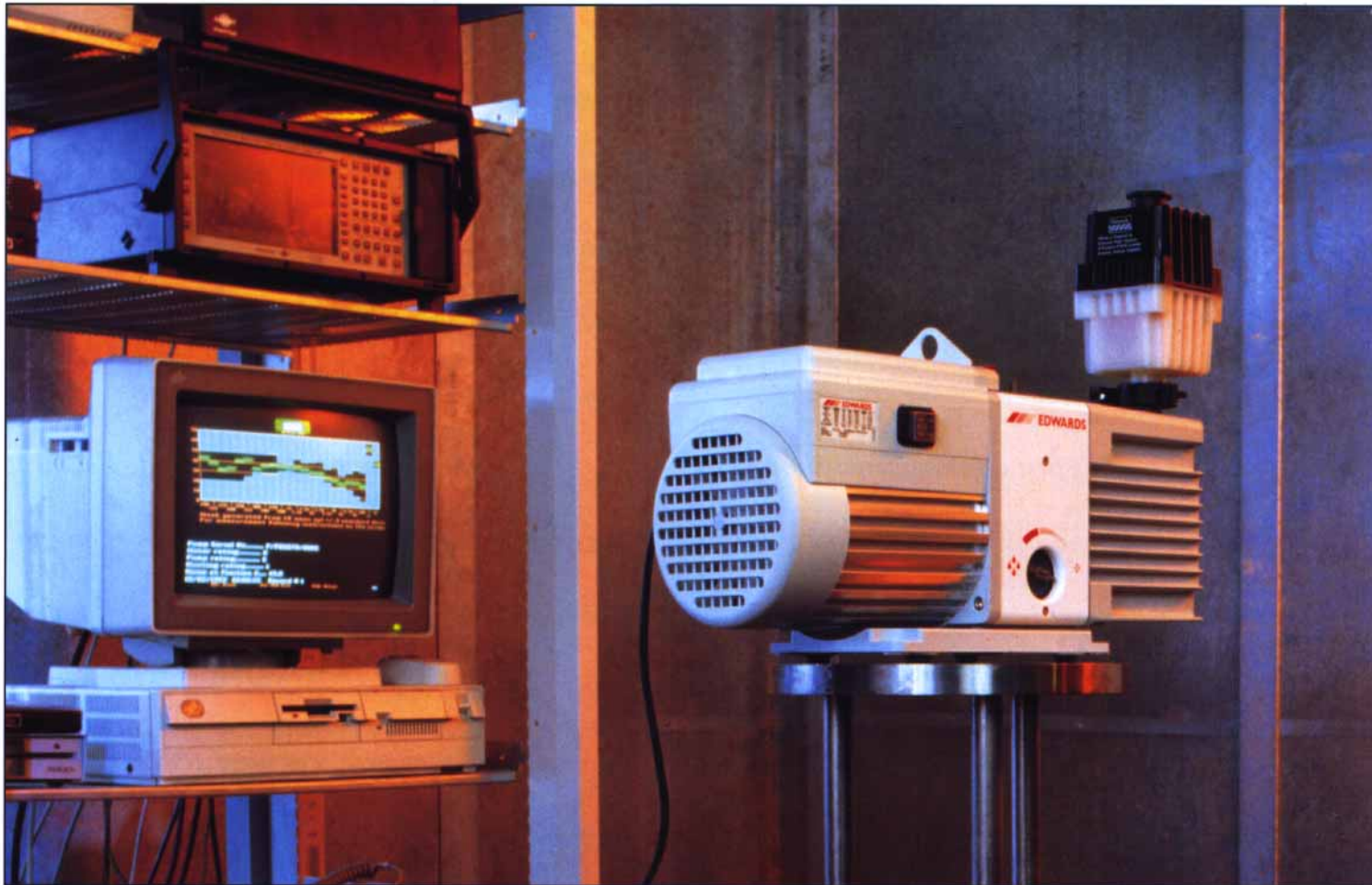
Each RV pump is noise tested in our quiet room using a noise spectrum analyser.
