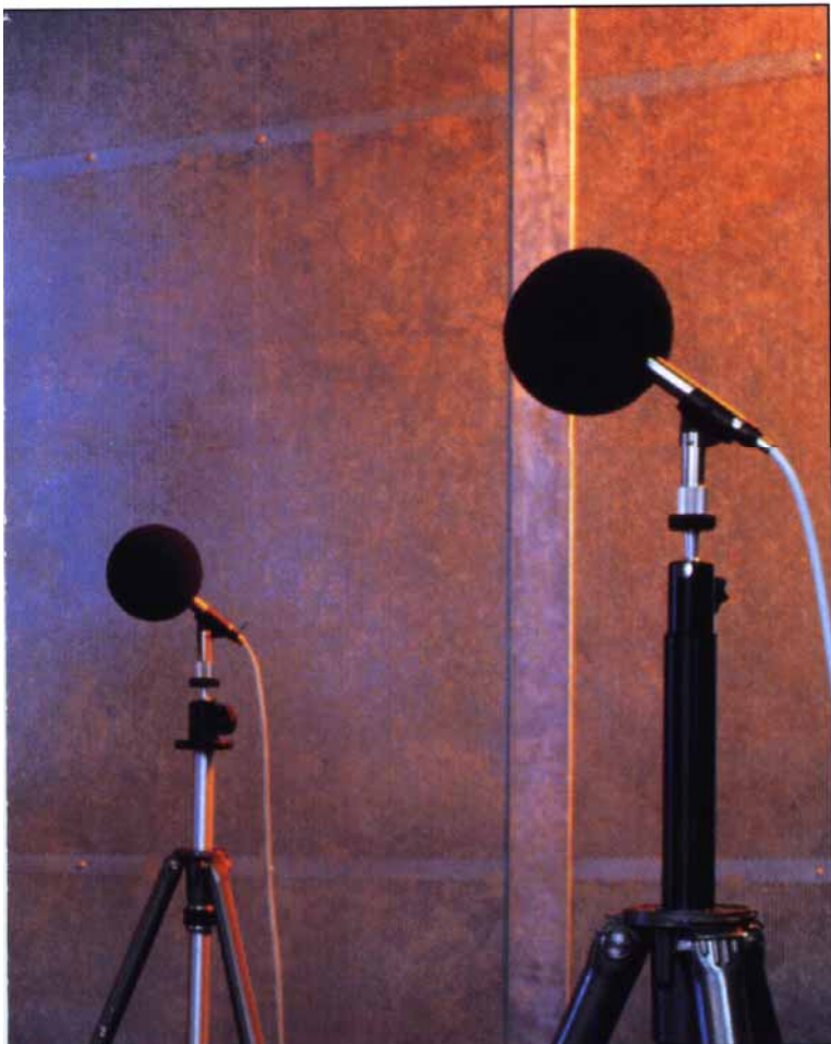
Noise levels of 48dBA are achieved. Individual frequencies must fall within the pass "mask" before a pump is released.
