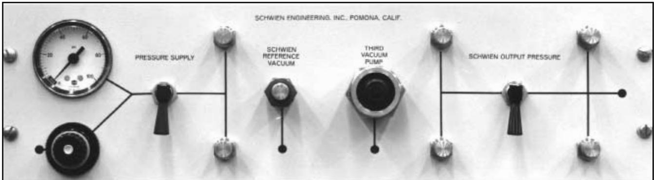
The **4541-1001 Pneumatic Service Panel** is designed to provide convenient connections for the Manometer's Output Pressure service to the various types of devices to be calibrated, tested, serviced, etc.
